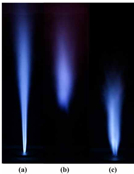
Fig. 3 Direct images of CH 4 /O 2 coaxial jet flames at NT: (O/F)_{mom} = 7.2 (a), 10.0 (b) and 28.0 (c) and Re_o = 6197-21149.
