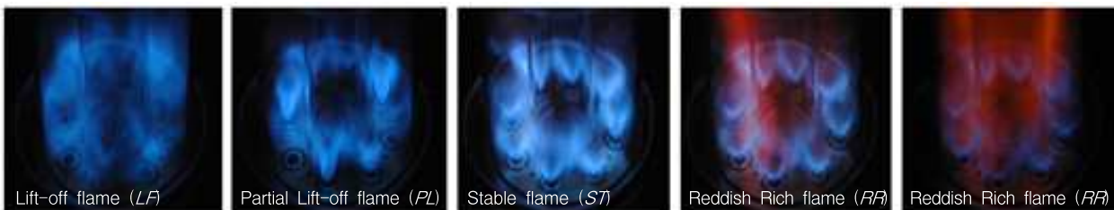
Fig. 3 Front view of the flame shapes according to the flame mode.
