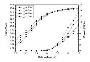
Figure 30. I-V characteristcs depending on oxide thickness
