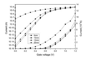
Figure 3. I-V characteristics varying by channel length
