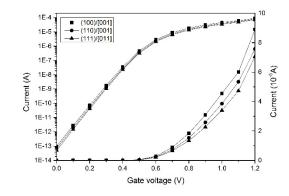
Figure 32 I-V characteristics varying crystal orientations
