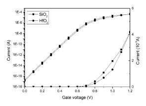
Figure 9. I-V characteris depending on oxide materials
