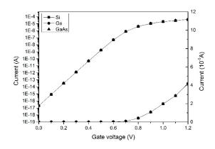
Figure 12. Wrong I-V characteristics from channel material simulations
