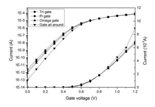
Fig. 2. I-V characteristics of multigate structures
