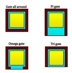
Fig. 1. Multigate FET structures
