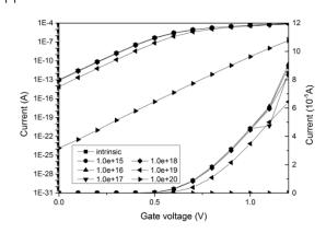
Figure 29. I-V characteristcs depending on channel doping concentration.
