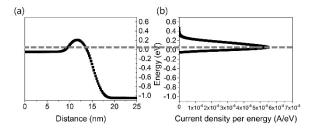
Figure 26. Tunneling phenomena observed at 10nm channel length
