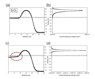
Figure 31. Source potential barrier lowered by fringing field
