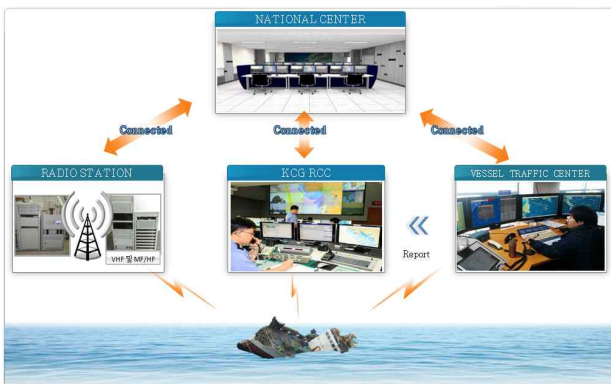
Fig. 9 International Safety Communication Center Operational Structure
