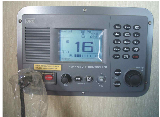
Fig. 3 VHF Radio Equipment
