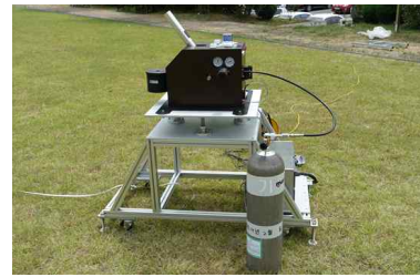
Fig. 3 Land test of heaving line launcher mock-up
