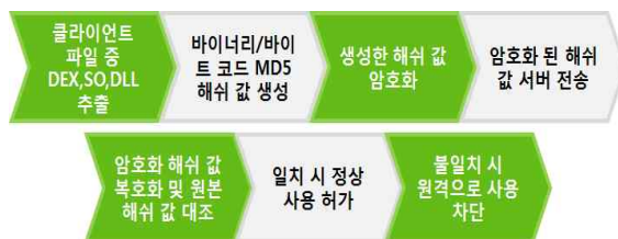
Integrity Check System Process
