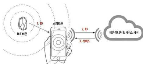
operation principle of the beacon
