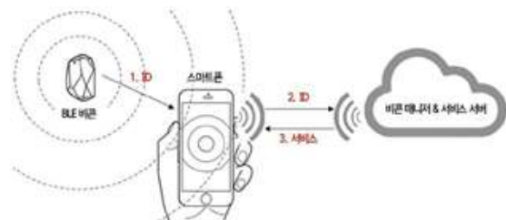
Fig. 1. BLE Beacon-based O2O System Architecture
