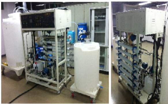
Fig. 2. Lab scale mobile high pressure RO system.
