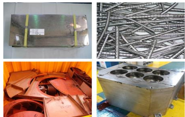
Fig. 2. Filter frame, Rebar, Storage vault, Exhaust fan (Clockwise from upper left).
