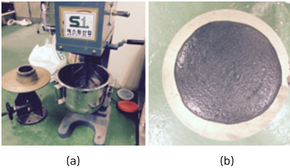
Fig. 1. (a) Cement mortar mixing apparatus and (b) workability test equipment.
