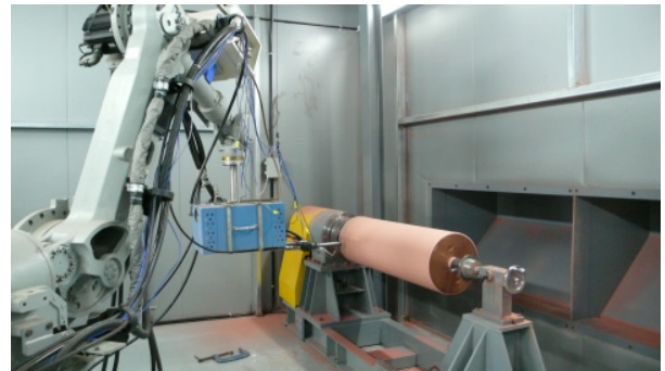
Fig. 4. Cold spray coating of Mid-scale cast iron container in the scale-up facility.
