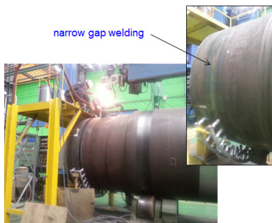
Fig. 1. KN-18 cask. Fig. 2. Welding on the cask body.
