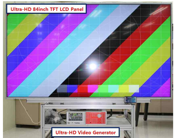
Fig 6. Ultra-HD Video Pattern using V-by-One HS Interface
