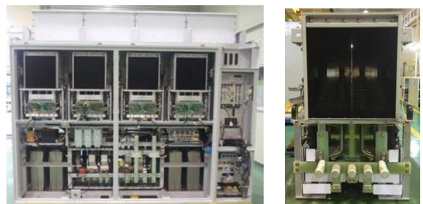
(a) 추진제어장치 (b) Inverter Stack
