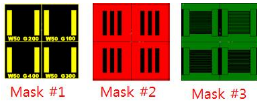
Fig. 3 Gold and silicon masks for gold deposition and silicon etching for micro capacitance sensor
