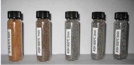
Fig. 3 Dyeing sludge ashes after reduction test
