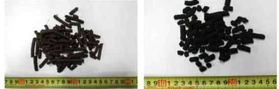
Fig. 9 Dyeing sludge + Rice husk Fig. 10 Dyeing sludge + Tar
