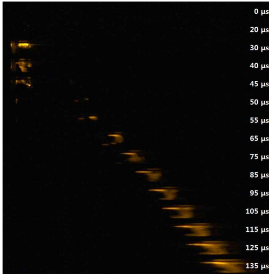
Fig. 5 Direct image for full region from rupture disk (rupture pressure 8.6 MPa)
