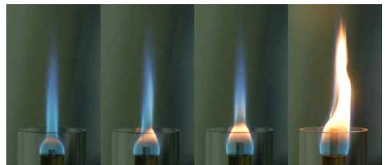
Fig. 5 Flame shape changes as the inner nozzle position increases.
