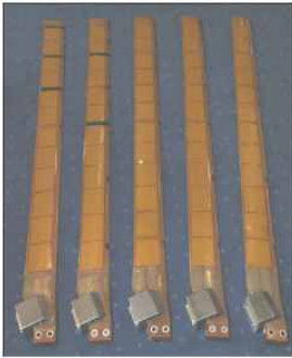
Figure 5 STAR Blades manufactured at DLR 8
