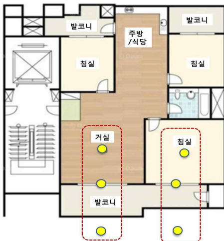
Figure 1 Noise measurement position of indoor and near by building
