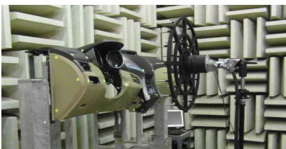
Figure 7 Sound Camera Array Setting
