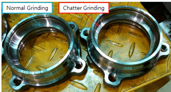
Fig.14 Normal vs chatter face after grinding process
