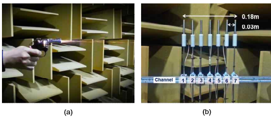
Fig. 4 Photographs of (a) generation of an impulsive sound using a gunshot and (b) a ULA with seven microphone elements (B&K ICP type-4935, reference microphone is channel 4).
