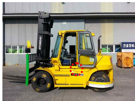
Fig. 2 Folk lift truck and motion measuring point
