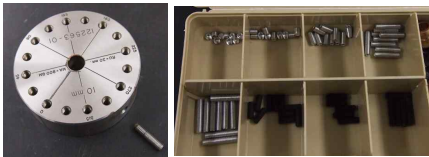
Fig. 3 Shape of disc and unbalance mass
