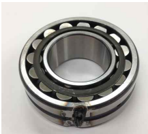
Figure 2 Bearing with outer race fault
