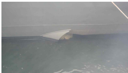
Fig. 4 Outlet of the exhaust for a diesel engine of a typical naval vessel
