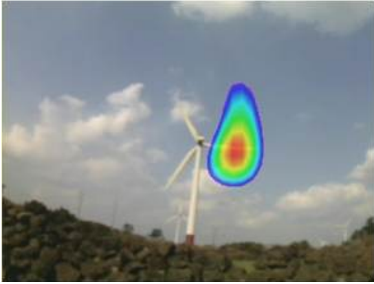
Fig. 7. Measured wind turbine noise source wind acoustic array system.
