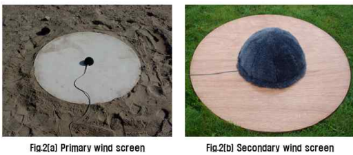
Fig. 2. Microphone and wind screen.
