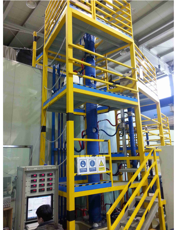
Fig. 4 Underwater acoustic performance measurement system(Pulse tube)
