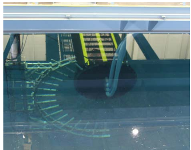
Fig. 3 Experiment setup for near field acoustic holography measurement
