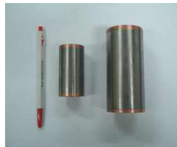
(a) Copper die casting rotor
