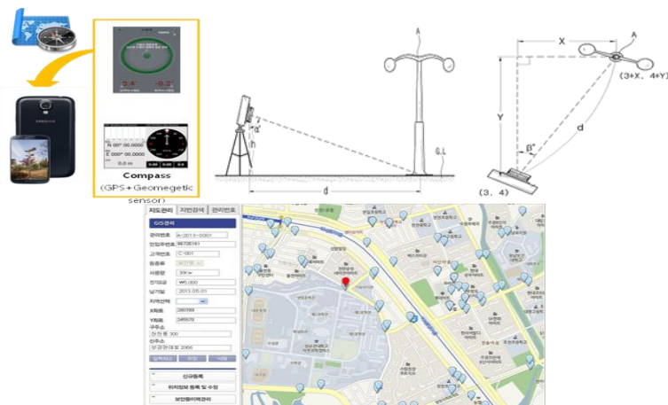
[Picture 1] Registration via mapping facility location and picture information on the map based on smart device application
