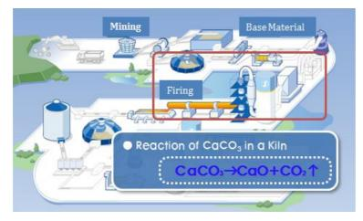
Fig.1 CaO<sub>2</sub> Emission from CaCO<sub>3</sub> during Cement Production by Fossil Fuel
