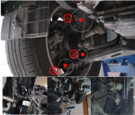
Figure 3. Position of accelerometer
