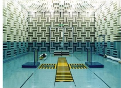
Figure 1. Semi-anechoic chamber
