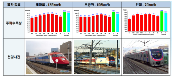
Fig. 5 Noise source characteristics of the vehicle
