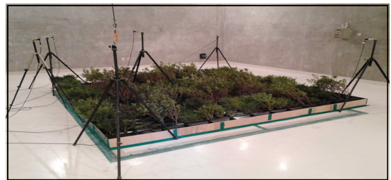
Fig 2. Measurement of sound absorbing coefficient
