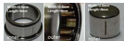
Figure 4. Kind of the defected bearing
