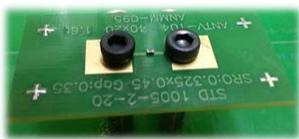
Figure 2 Fixed condition of MLCC on the circuit board
