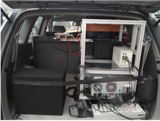
Fig.5 Set up for active interior noise control Instrument based on new adaptive algorithm of the FXLMS
