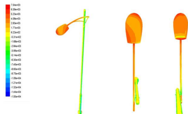
Fig. 5 The pressure distribution for maximum 45 degree direction wind load
