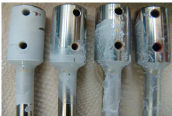
Fig. 3 Initial crack location
