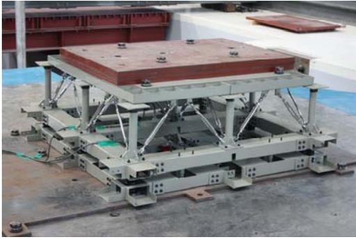
Photo 1 Shake table test of vertical isolator
