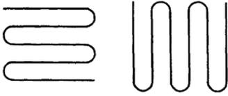
Fig. 2 Example of a scanning Pattern
