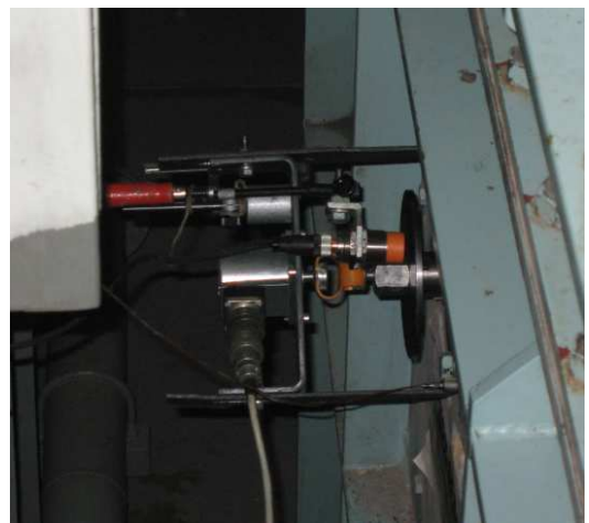
Fig.14 Torsional Vibration Measurement Equipment at Fore side
