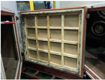
Fig. 3 Installed 4 x 4 cell panel with unit cell size of 205 mm x 255 mm.
