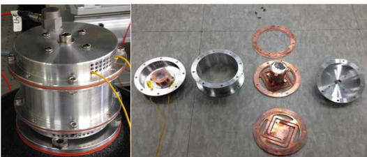
Figure 3 Assembly and components of the energy harvester
