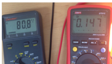
DC LED 전압 : 80.8Vdc/전류 : 0.147 P : 11.76W
