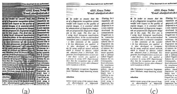
Fig. 2. (a)Result of first binary; (b)Result after run length histogram technique(with horizontal and vertical pattern width are 2); (c)Result after masking from input image.
