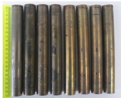
Fig. 2. The specimens of defected steam generator tube
