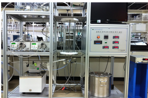
Fig. 1. The system for the chemical cleaning
